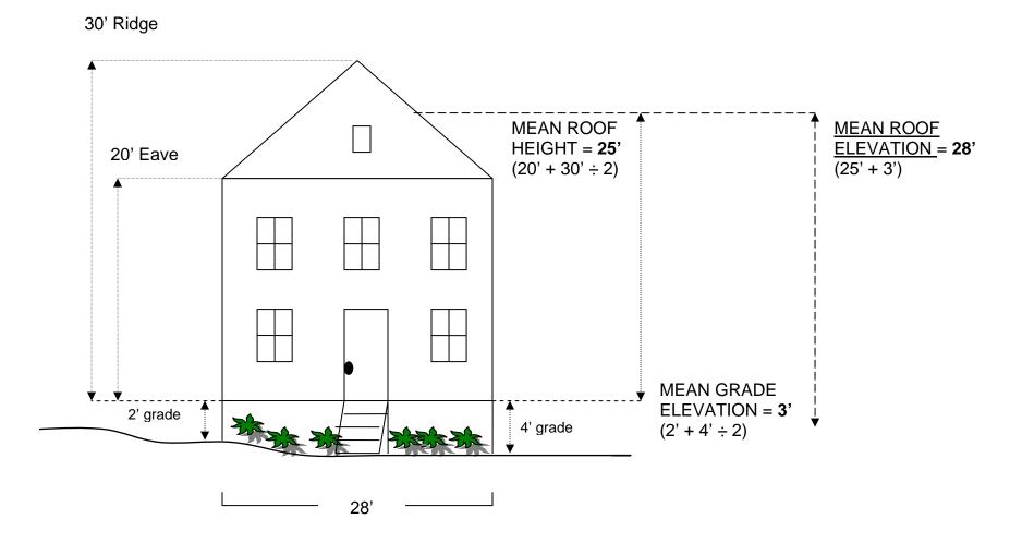
Roof height (or mean roof elevation) is measured from the **mean grade elevation** (average grade around the perimeter of the building, or in this example,  $2' + 4' \div 2 = 3'$ ) to the **mean roof height** (one-half the vertical distance from the eave to ridge, or in this example,  $30' + 20' \div 2 = 25'$ ).
