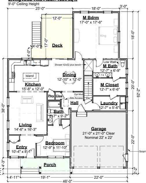
First Floor Plan Scale: 3/32" = 1'-0"
